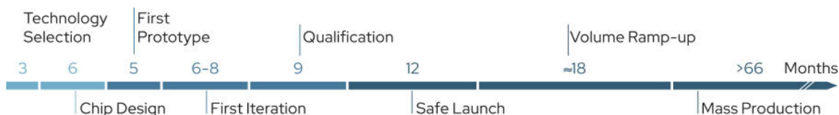
Fig. 4.5: Illustrative lifecycle for automotive: Analog/mixed-signal products are much more specialized for their applications and are used for many years
