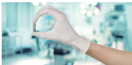
Fig. 4.14: X-FAB manufactures an application-specific integrated circuit (ASIC) for usage in leadless pacemakers
